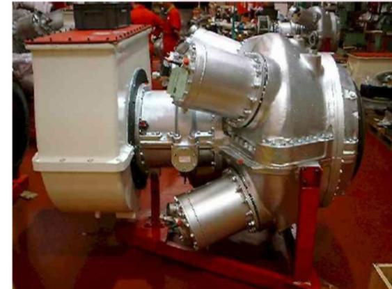
A gas turbine consists of a compressor, combustor, and power turbine.
